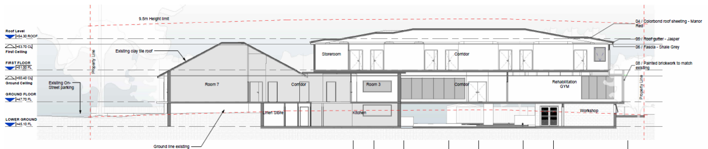
Figure 21 – Proposed Excavation to Extend the Lower Ground Level and to Create a Newly Introduced Three Storey Component (New Works in White/Existing Facility Shaded in Grey)
